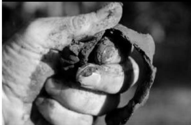
Figure 1: Making a soil ribbon
